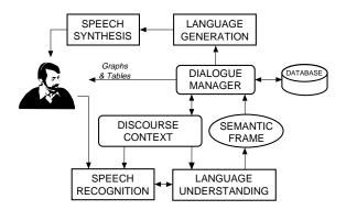
Figure 1: Block diagram of a spoken dialogue system.
