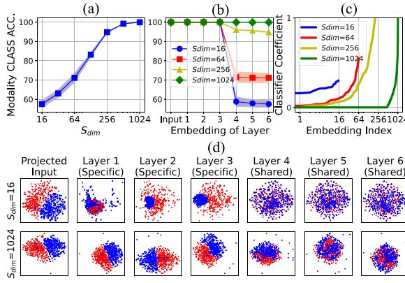
Fig. 3. (a) Modality classification accuracy based on the last layer representation of UAVM with various  $S_{dim}$ . (b) Modality classification accuracy based on intermediate representations of each layer of UAVM models. (c) The sorted modality classifier coefficients. (d) t-SNE plot of the intermediate representations of each layer with audio input (red) and video input (blue).
