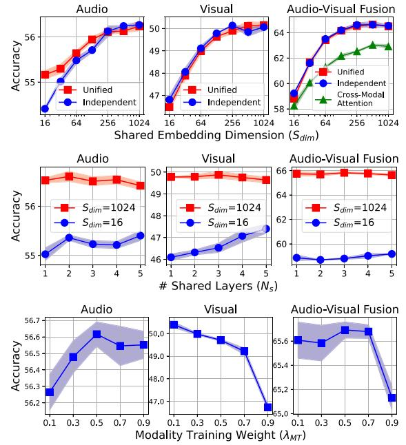
Fig. 2. The audio-based, video-based, and fused accuracy on VGGSound with various shared embedding dimension  $S_{dim}$  (upper), number of shared layers  $N_s$  (middle), and modality training weight  $\lambda_{MT}$ .
