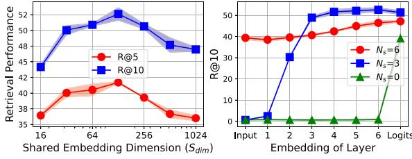
Fig. 4. (Left) A-V retrieval performance based on the last shared Transformer layer representation of UAVM models ( $N_s = 3$ ) with various shared embedding dimensions  $S_{dim}$ . (Right) A-V retrieval performance based on the representation of various layers of models with  $N_s = 0$  (fully independent model),  $N_s = 3$ , and  $N_s = 6$  (fully unified model) and  $S_{dim} = 128$ .
