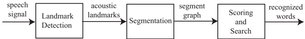
Figure 1-1: Block diagram of a segment-based speech recognition system
