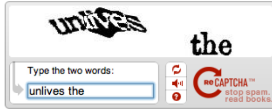
Figure 2-2: ReCAPTCHA digitizes books and secures websites simultaneously. A user attempting to access a ReCAPTCHA -secured site is presented two digitally scanned words which they must transcribe. One of the words, the “control” word, is known to the algorithm and is used to verify that the user is human. The transcription of the other is compared across other users given the same word. Their agreement is used to transcribe this previously unknown word.
