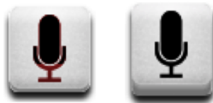
Figure 3-5: Example of a traditional speech recording interface: user presses once to record and once to stop recording. Button is highlighted red (left) to indicate that system is in record state.
