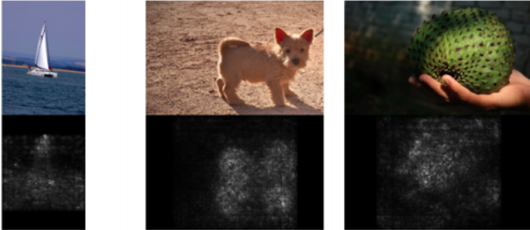
Figure 2-4: An example of pure gradients being used to provide transparency on an image classification task. We can observe that the larger gradients (bottom) correspond to the regions of the original images (top) that contain the object of interest (Simonyan et al., 2014).
